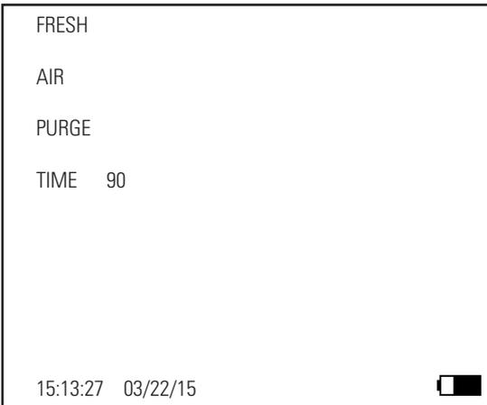
The time will count down in seconds to zero and is pre-set by the analyzer. During countdown the analyzer will initialize the measuring system, do not block the end of the probe or insert into or near the vehicle exhaust. It also displays some setup values including atmospheric pressure and internal ambient temperature.
